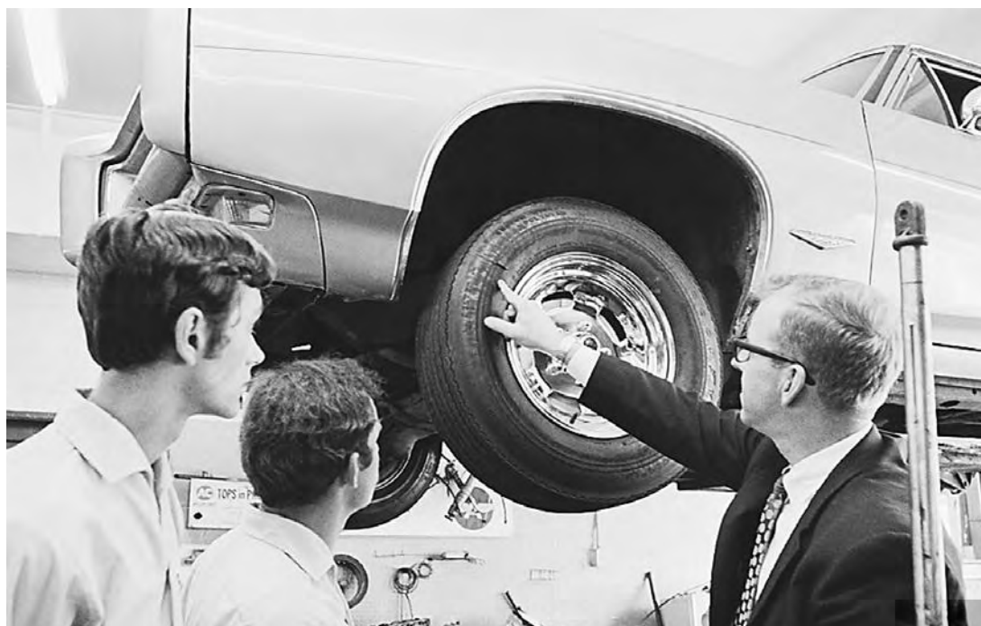
THE HYDRAULIC PRESS, LIKE THE LIFT HOLDING UP THIS CAR IN A REPAIR SHOP, IS A RELATIVELY RECENT INVENTION THAT IS USED IN MANY MODERN DEVICES, FROM CAR JACKS TO TOILETS. (Photograph by Charles E. Rotkin/Corbis. Reproduced by permission.)
