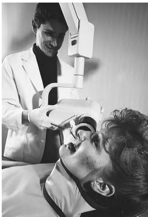
“SOFT” X-RAY MACHINES, SUCH AS THIS ONE BEING USED BY A DENTIST TO PHOTOGRAPH THE PATIENT’S TEETH, OPERATE AT RELATIVELY LOW FREQUENCIES AND THUS DON’T HARM THE PATIENT. (Photograph by Richard T. Nowitz/Corbis. Reproduced by permission.)
