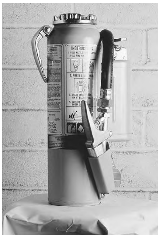
A FIRE EXTINGUISHER CONTAINS A HIGH-PRESSURE MIXTURE OF WATER AND CARBON DIOXIDE THAT RUSHES OUT OF THE SIPHON TUBE, WHICH IS OPENED WHEN THE RELEASE VALVE IS DEPRESSED. (Photograph by Craig Lovell/Corbis. Reproduced by permission.)
