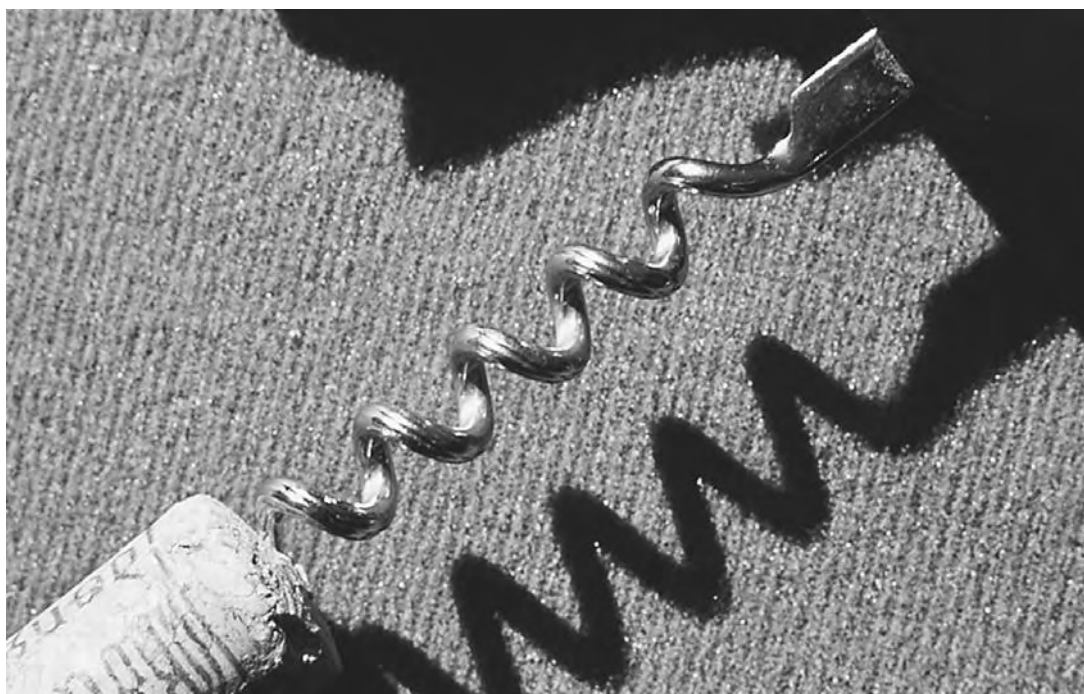
A SCREW, LIKE THIS CORKSCREW USED TO OPEN A BOTTLE OF WINE, IS AN INCLINED PLANE IN THE SHAPE OF A HELIX, WRAPPED AROUND AN AXIS OR CYLINDER. ( Ecoscene/Corbis. Reproduced by permission. )
