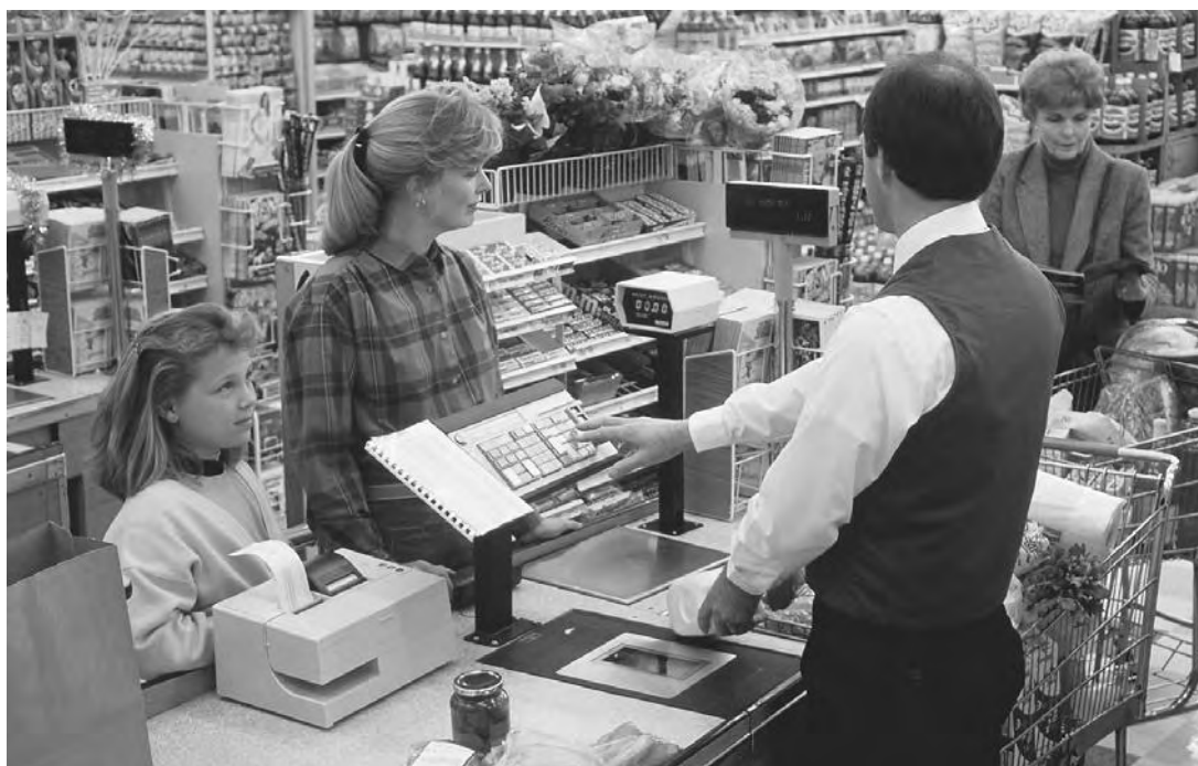
THE CHECKOUT SCANNERS IN GROCERY STORES USE HOLOGRAPHIC TECHNOLOGY THAT CAN READ A UNIVERSAL PRODUCT CODE (UPC) FROM ANY ANGLE. (Photograph by Bob Rowan; Progressive Image/Corbis. Reproduced by permission.)
