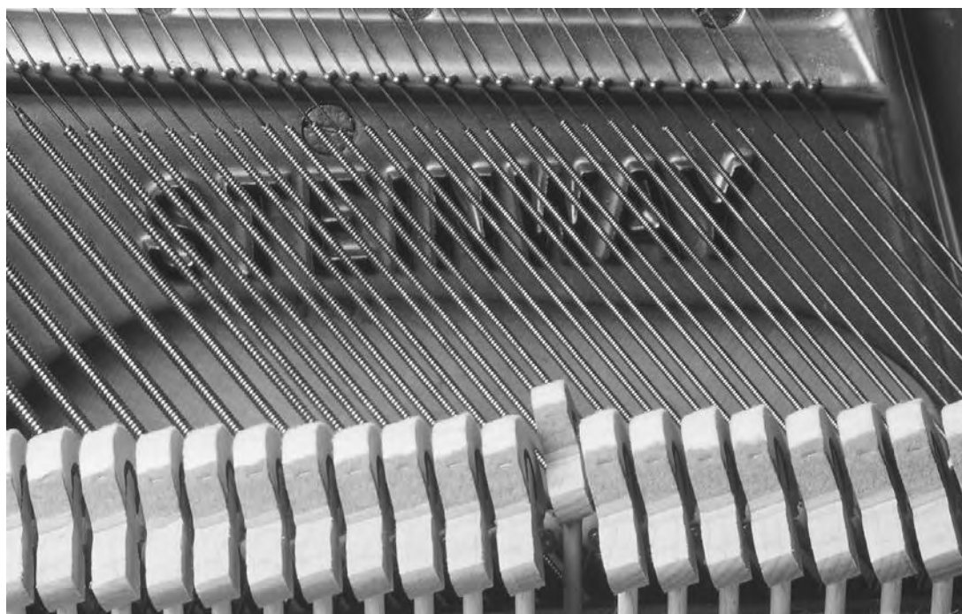
PIANO STRINGS GENERATE SOUND AS THEY ARE SET INTO VIBRATION BY THE HAMMERS. THE HAMMERS, IN TURN, ARE ATTACHED TO THE BLACK-AND-WHITE KEYS ON THE OUTSIDE OF THE PIANO. (Photograph by Bob Krist/Corbis. Reproduced by permission.)
