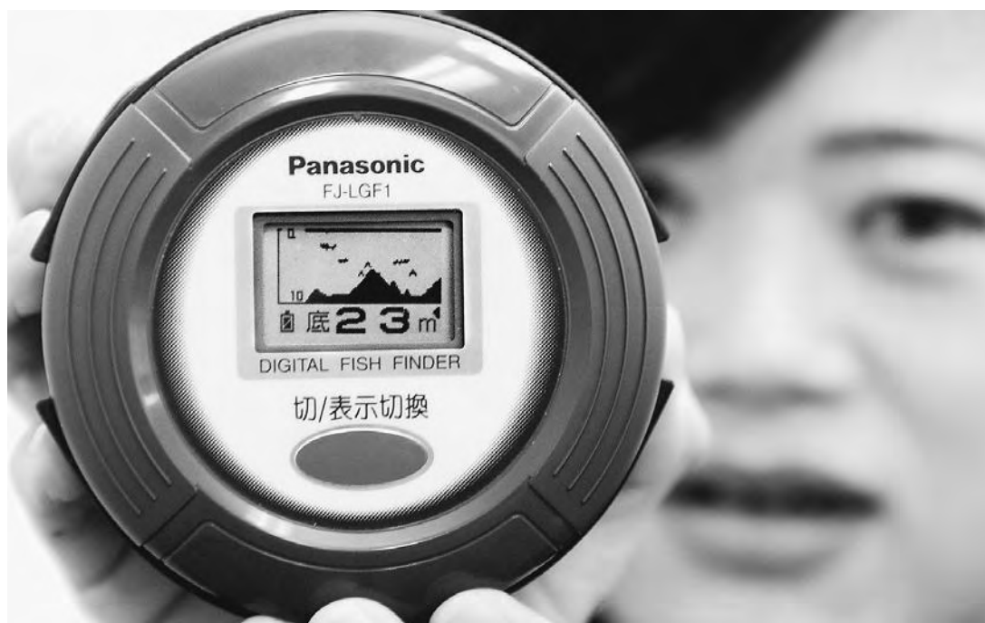
A FISHING REVOLUTION? IT'S POSSIBLE, THANKS TO THIS ELECTRONIC FISH-FINDER DEVELOPED BY MATSUSHITA. THE DEVICE INCLUDES A DETACHABLE SONAR SENSOR. (AFP/Corbis. Reproduced by permission.)
